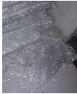
Gambar 1. Fiberglass jenis Chopped Strand Mat
